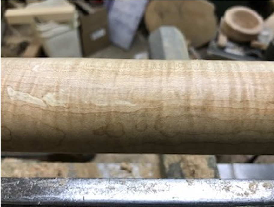
Photo 1) finish directly from skew chisel plane cut on the lathe (no sanding, straight from the chisel).
