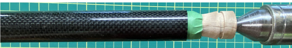
Figure 7. The spurtle was glued together, placed in the carbon fiber tube and pressed together between centers on the lathe.
