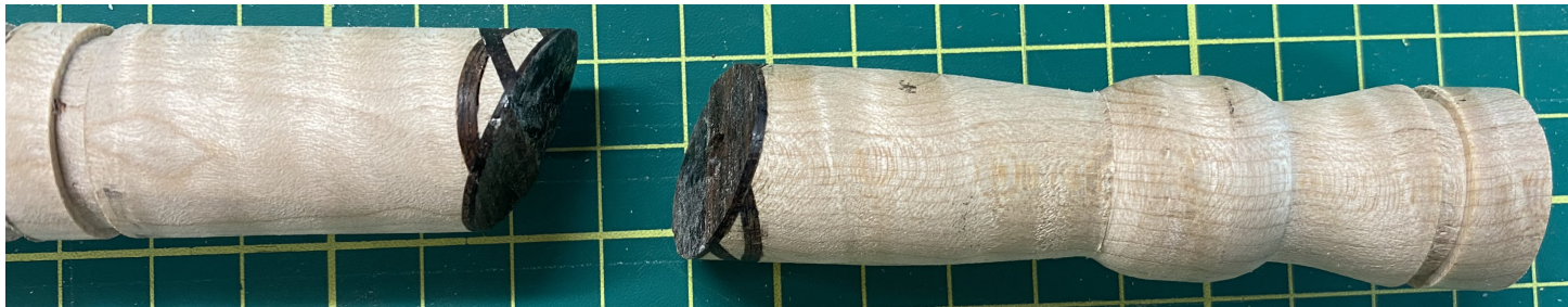
Figure 1. A failed Celtic Knot on a spurtle under construction... One of the lamination glue lines failed while on the lathe.
