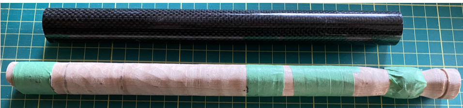
Figure 3. The spurtle shaft had masking tape used to increase the diameter of the shaft to fit snugly in a section of carbon fiber tube.
