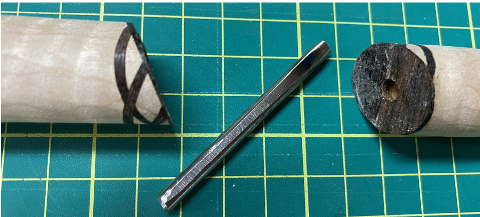
Figure 6. The \frac{3}{16} " diameter repair pin with a flat ground into one side to facilitate glue-ing, preventing air locks.
