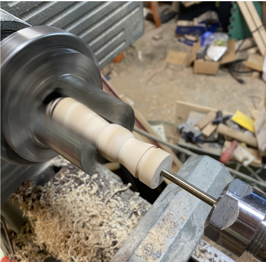
Figure 2. The broken end of the spurtle was mounted in pen jaws and drilled out on the lathe.
